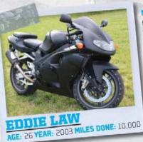
MODS: Pipercross air filter, stubby cans, Yoshimura box map, heated grips, truck bedliner coating on body and frame, sliders, additional brake light **BEST UPGRADE:** "Heated grips—I ride year round." FAVORITE ASPECT:
